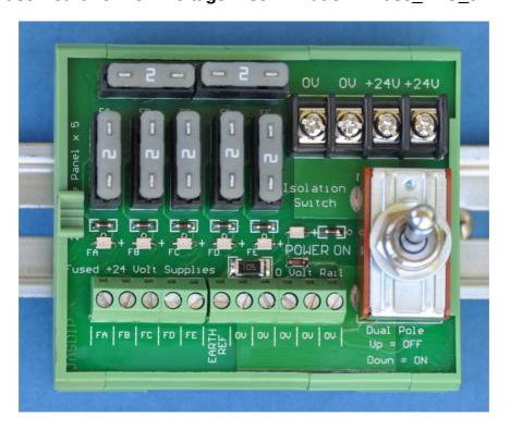
24VDC Control power supplies are typically current limited. If a fault occurs on the 24VDC line then the power supply lowers its output voltage to a safe current limit. This makes fault finding which device on the supply line has failed a trial and error task. By breaking up the supply with low voltage fuses, fault finding discrimination is improved.
